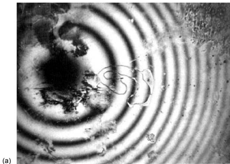
FIGURE 8 The interference pattern of 8-OCB (wavelength \lambda = 546 nm, magnification 90 \times ): (a) in the nematic phase at 77°C; (b) in the solid state at 35°C, (c) the temperature dependence of the birefringence \delta n for 8-OCB in the nematic, smectic A, and crystal phases measured using the proposed method. The solid line presents the fitting of \delta n to Equation (11) in the nematic phase.
